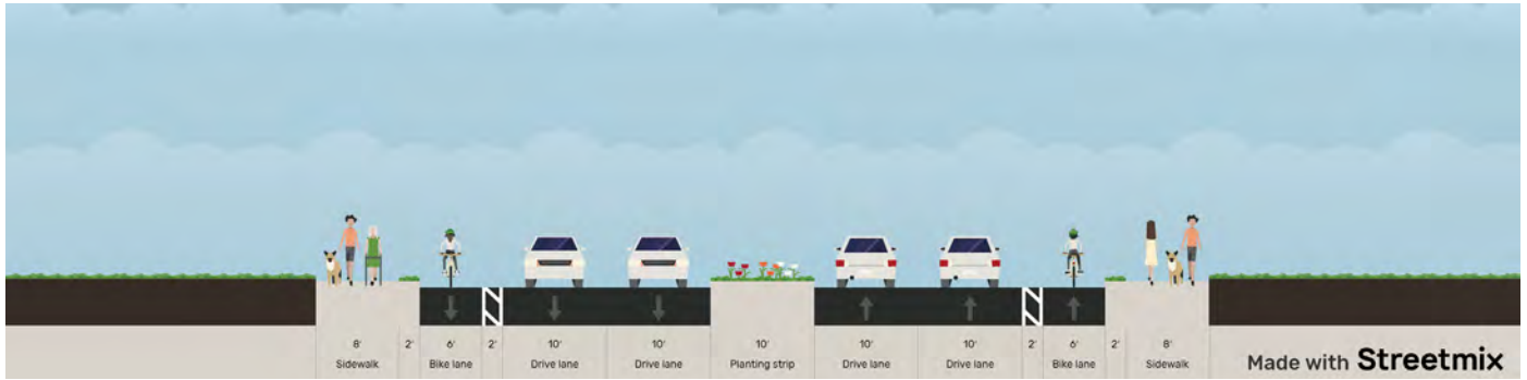
Figure 53: Proposed Cross Section for 104th Avenue
