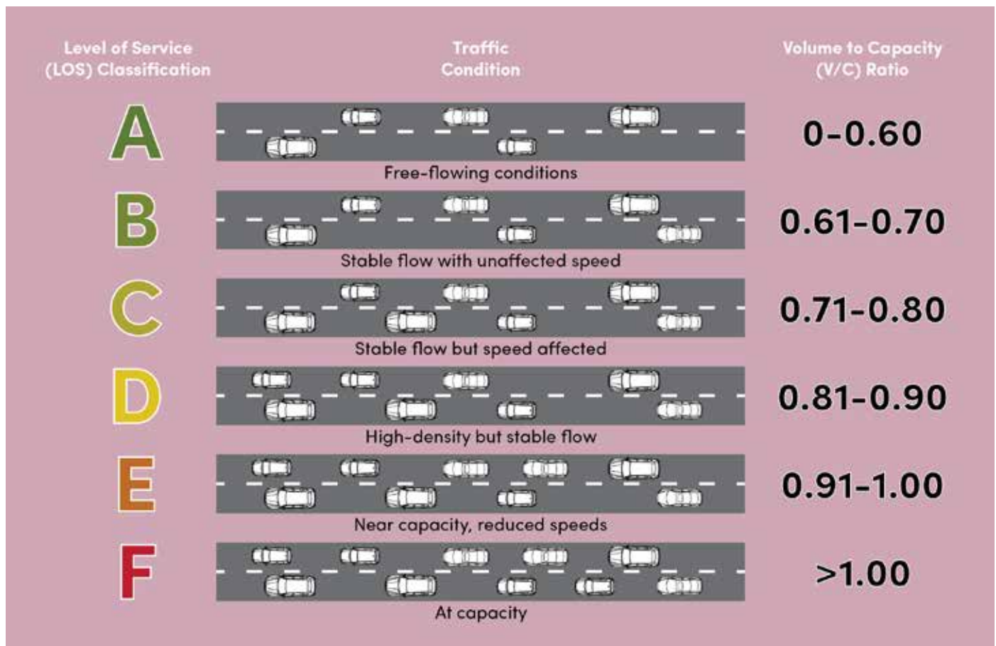
Figure 2.5: Level of Service and Volume to Capacity Ratio Concept (source: Fehr & Peers)
