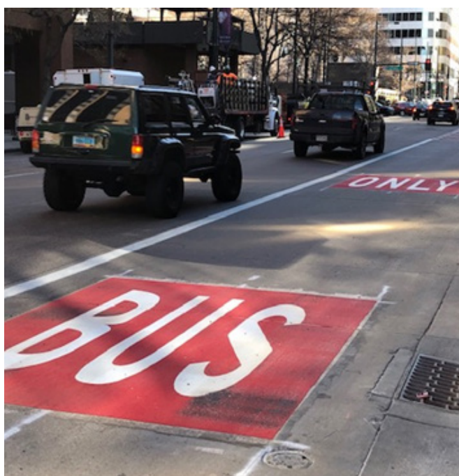
Figure 2.6: Example of a Dedicated Bus Lane in Downtown Denver (source: Fehr & Peers)
