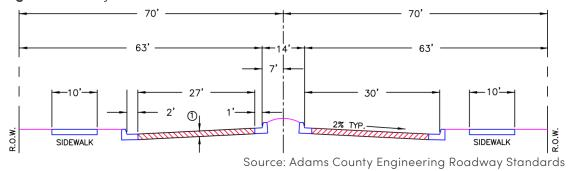
Figure 3.3: Enhanced Multimodal Corridor Arterial Cross Section
