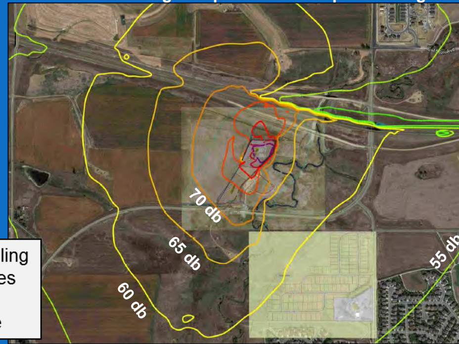
Noise during Completions – with partial mitigation
