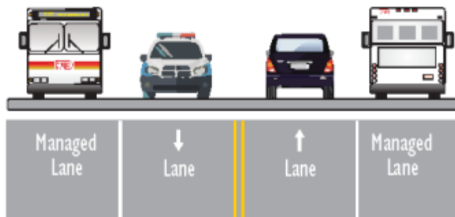
Figure 3.1 Managed Lane Cross-Section
