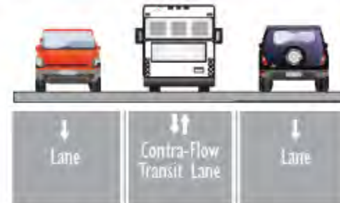
Figure 3.2 Reversible Transit Lane Cross-Section
