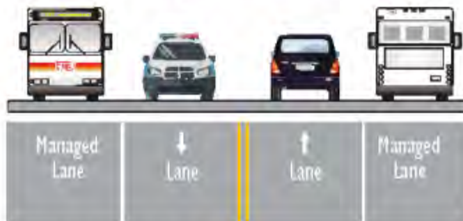
Figure 3.1 Managed Lane Cross-Section
