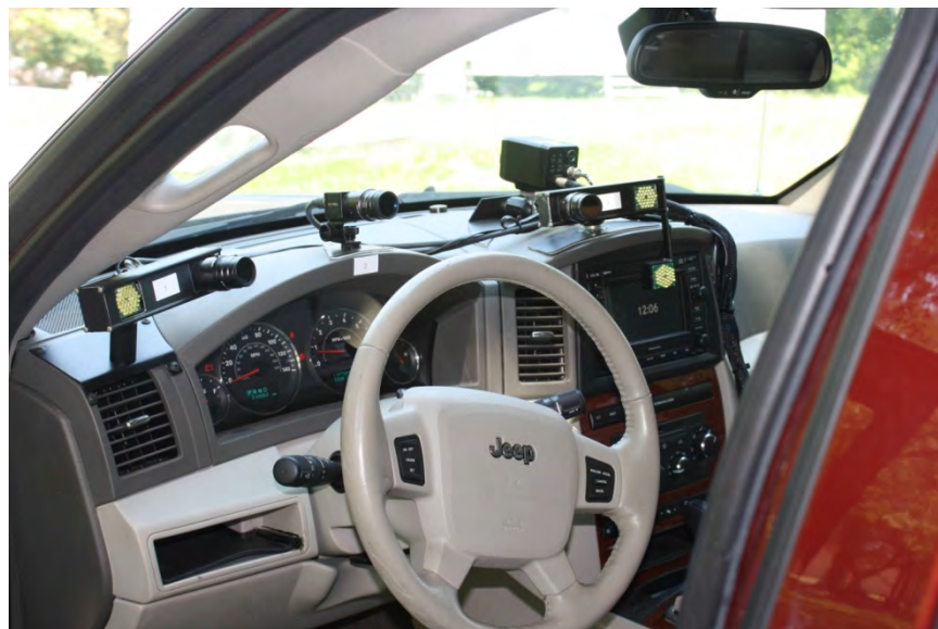
Figure 1. Smart Eye Face Camera Placement.
