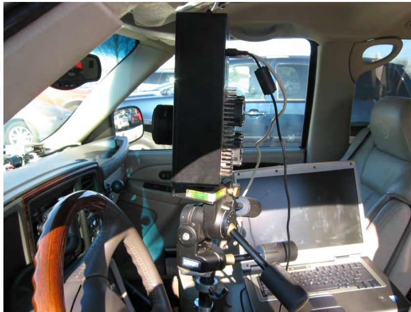
Figure 3. CCD Photometer and Laptop Setup in Vehicle
