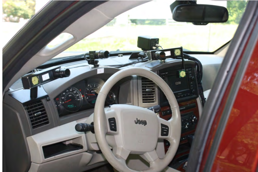
Figure 1. Smart Eye Face Camera Placement.
