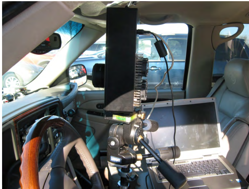
Figure 3. CCD Photometer and Laptop Setup in Vehicle
