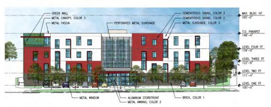
PDP elevation facing Broadway (east elevation)
