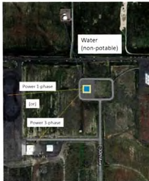
Figure 4 – Test Cell Location – Relative to Power & Water Sources
