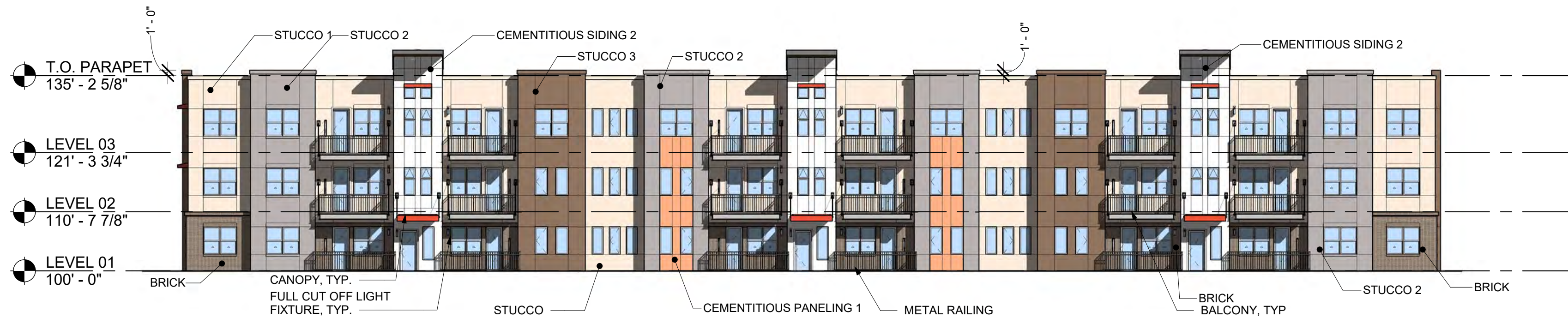
1 BUILDINGS 1 & 2 PARKING SIDE ELEVATION SCALE: 1/16" = 1'-0"
