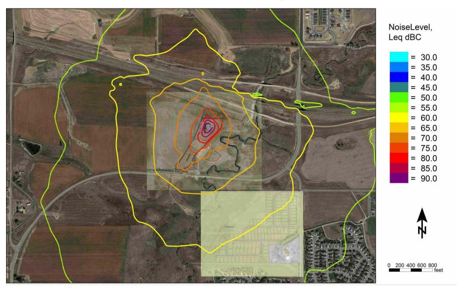
Figure 4-18 Mitigated Drilling Location 1 Noise Contour Map (dBC)
