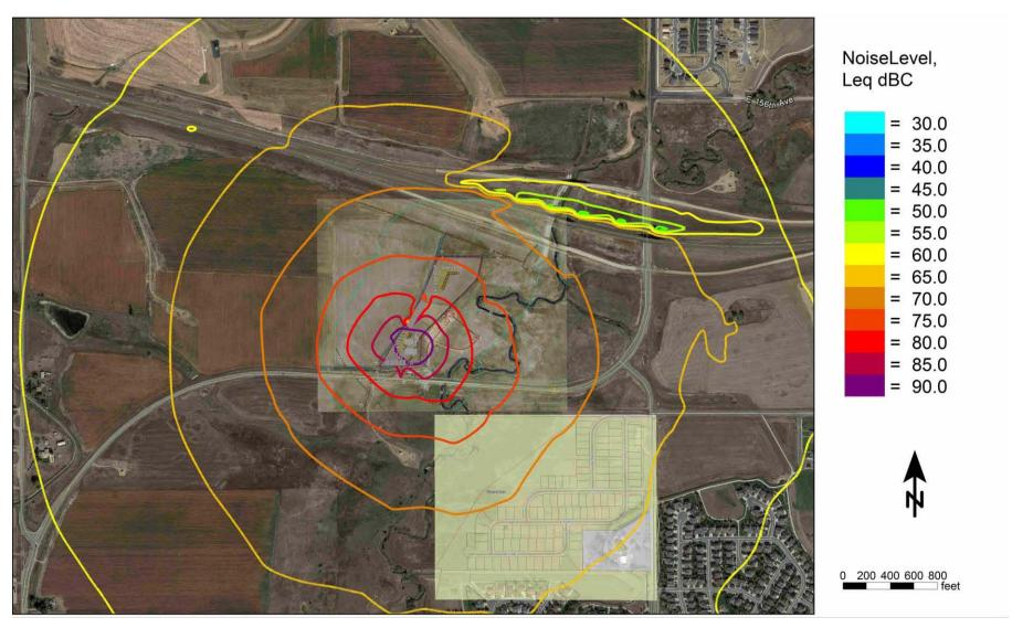
Figure 4-12 Unmitigated Fracing Location 2 Noise Contour Map (dBC)
