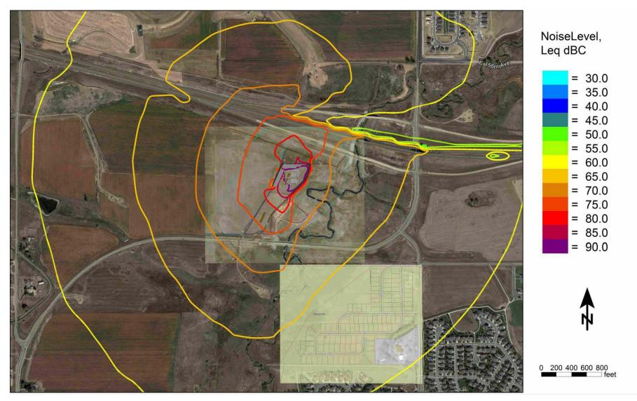
Figure 4-22 Mitigated Fracing Location 1 Noise Contour Map (dBC)
