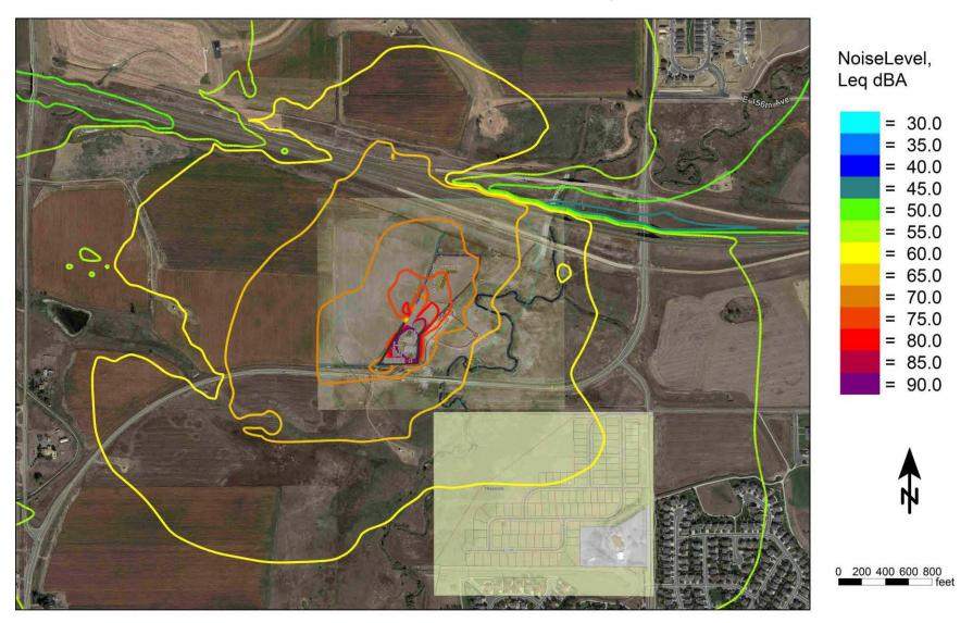
Figure 4-23 Mitigated Fracing Location 2 Noise Contour Map (dBA)
