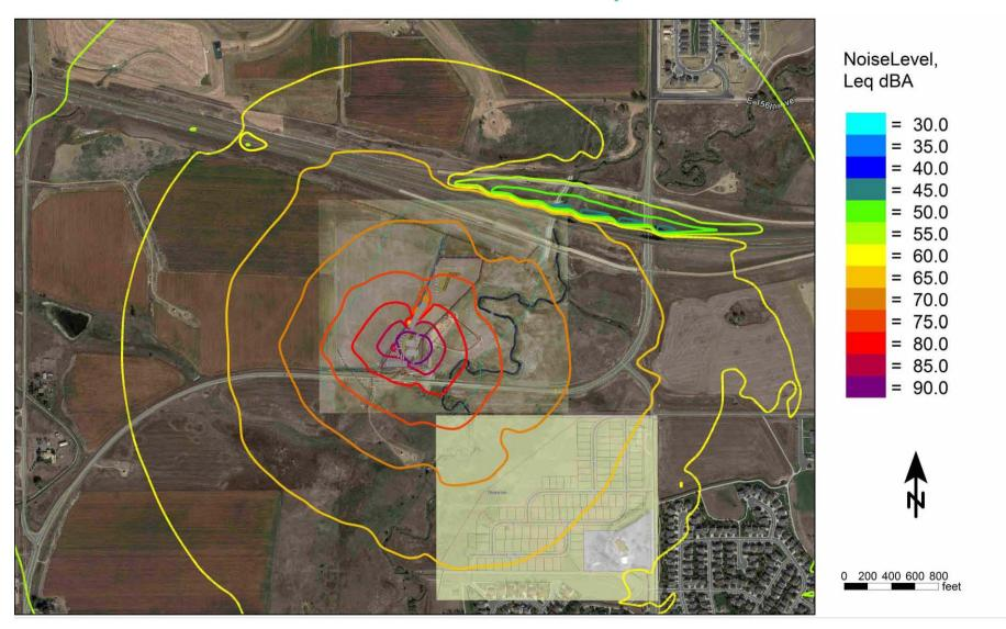
Figure 4-11 Unmitigated Fracing Location 2 Noise Contour Map (dBA)
