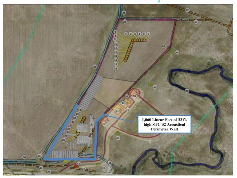
Figure 4-16 Modeled Mitigated Fracing Scenario Layout Location 2
