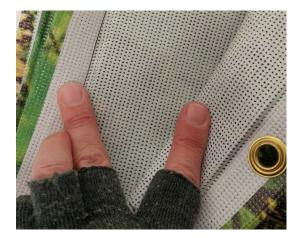
FIGURE 5. DERRICK WRAP MATERIAL.
