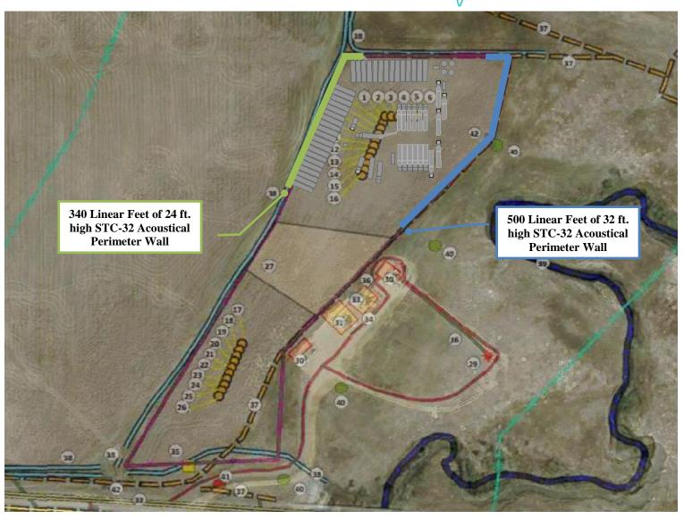
Figure 4-15 Modeled Mitigated Fracing Scenario Layout Location 1
