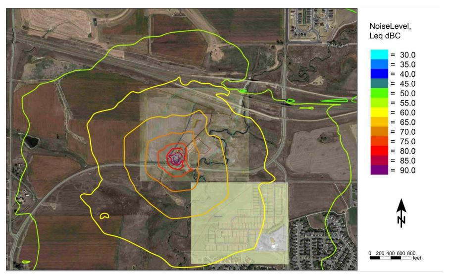
Figure 4-8 Unmitigated Drilling Location 2 Noise Contour Map (dBC)
