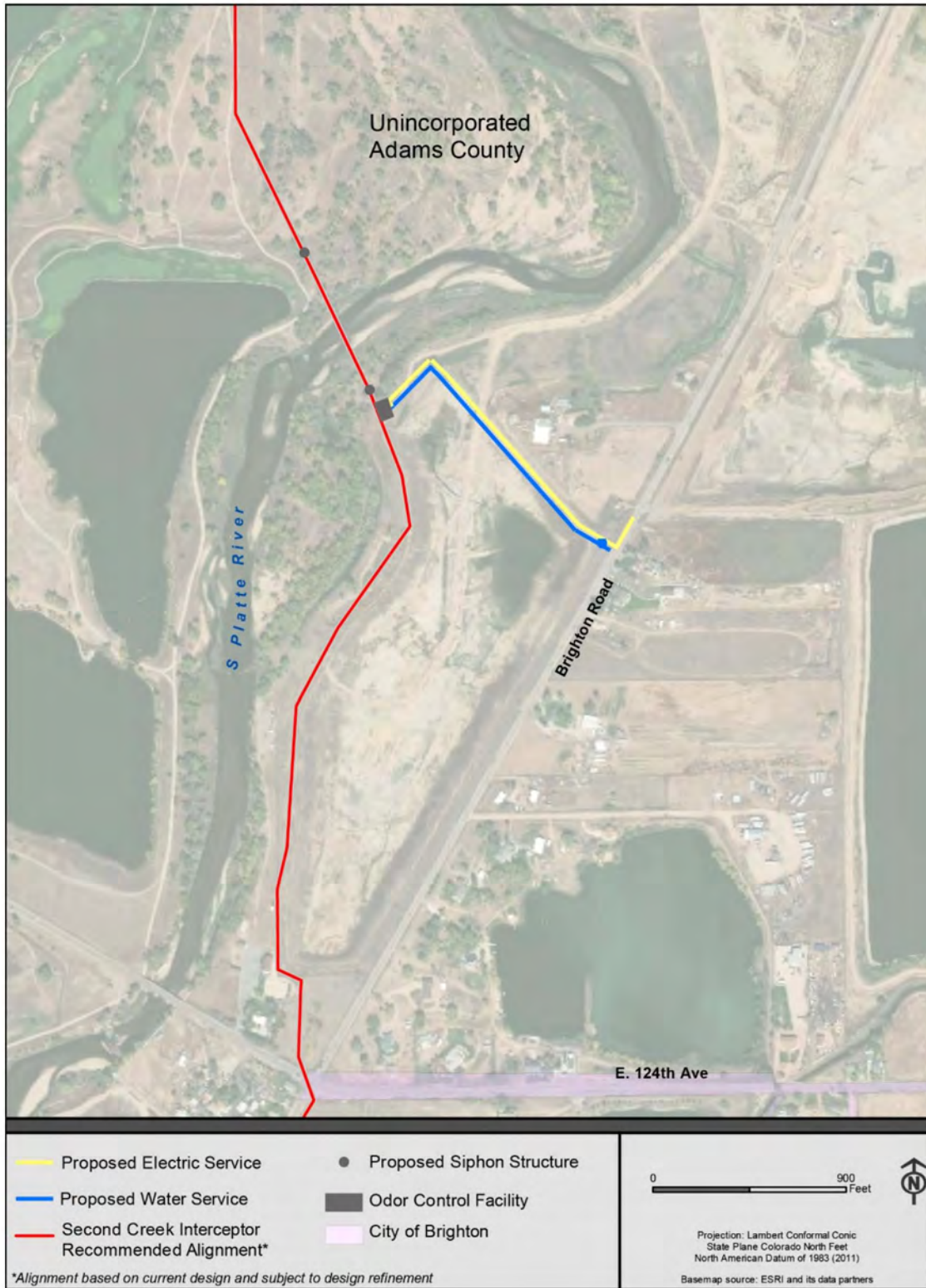
Figure 1-7: Odor Control Facility
