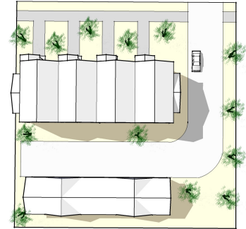
Fig. 3-276-H: Perimeter Street Orientation
