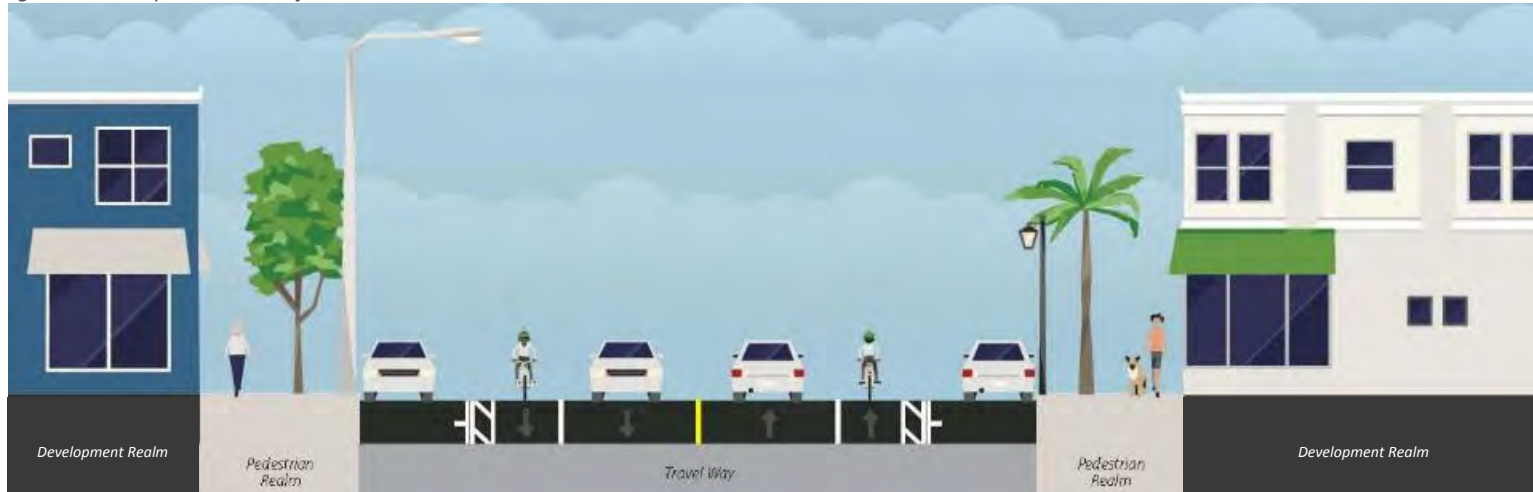
Figure 4-4: Component Parts of a Street
