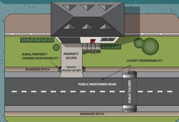
Roadside ditch maintenance responsibilities should be determined by Plat. Per Adams County Development Standards and Specifications Section 8-01-06, Table 8.7: maintenance of the access and drainage improvements within county right of way shall be the responsibility of the adjacent property owner.
