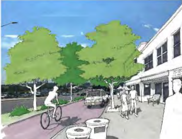
A sketch showing the same sidewalk with 'boulevard' street cross section implemented. Buildings are closer to the street, curbs are eliminated, service lane with parking buffers the pedestrians from the faster flowing traffic on Federal.
