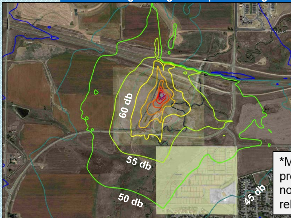
Noise during Drilling – with partial mitigation
