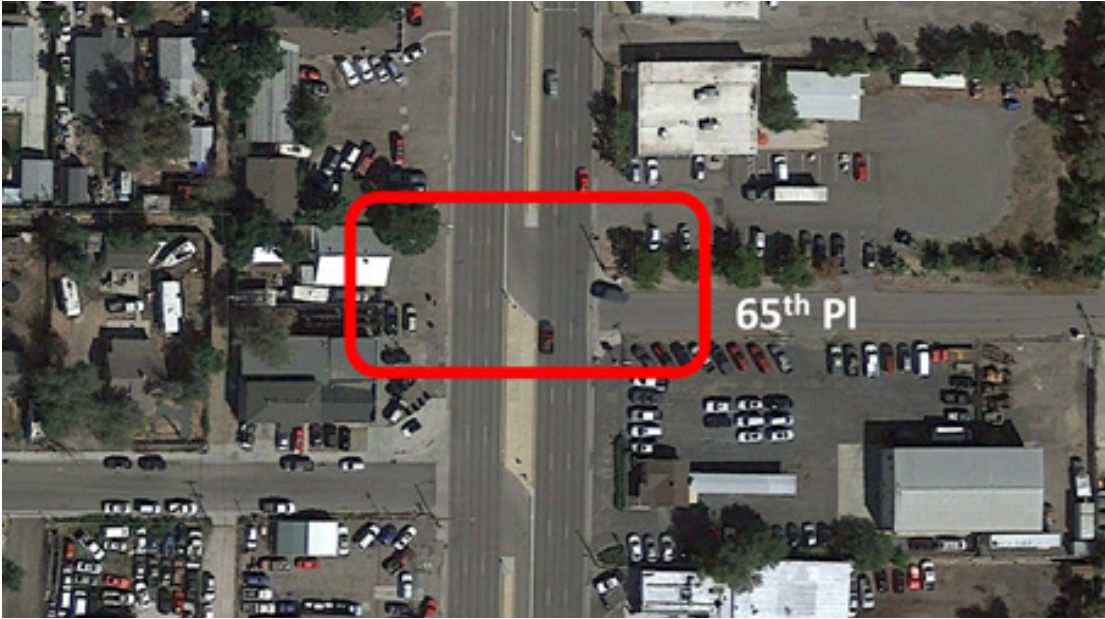
Figure 35: Example of an Opportunity for Adding Pedestrian Crossing Treatments on Federal Boulevard
